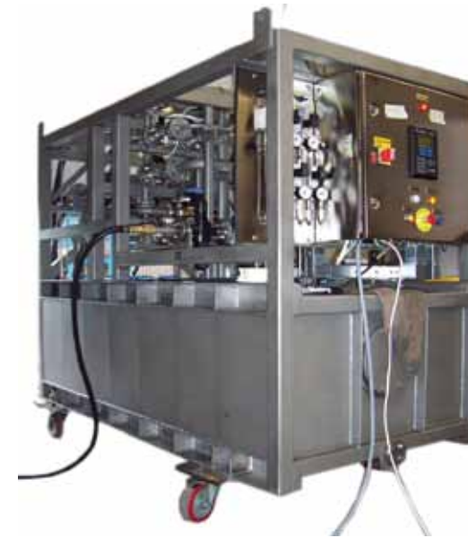
Rochem manufactures simple to highly sophisticated compressor wash skids such as this system for the UK's latest warships which is built for shock loadings of 25G
